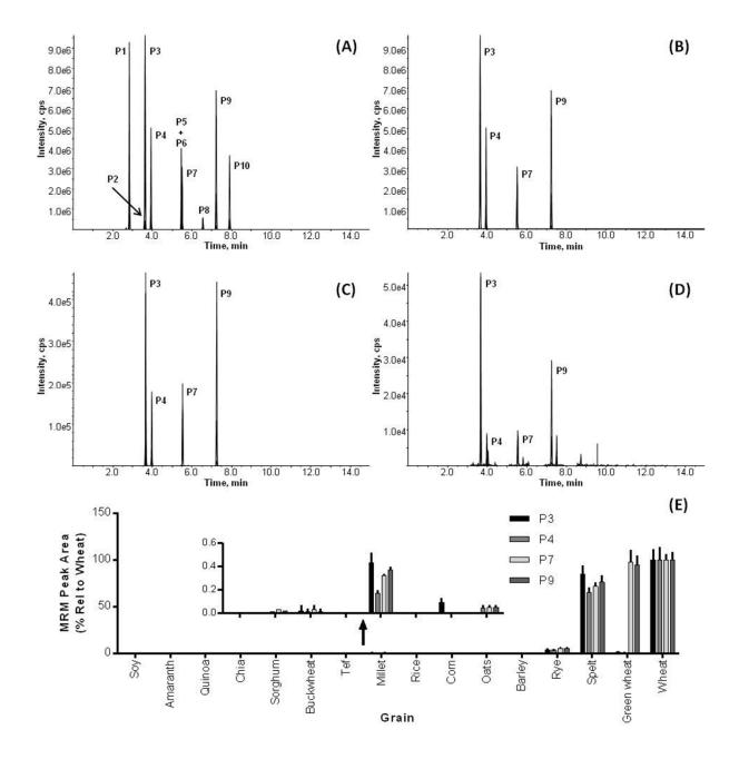
**Figure 2.** From the top 10 wheat-specific peptide markers (A), the best 4 were selected (B) and allowed the detection of wheat contamination in rye (C) and millet (D) flour. Detection of contamination in commercial products: (E) Flour from rye, millet, sorghum, buckwheat, and oats were confirmed with low level wheat contamination
